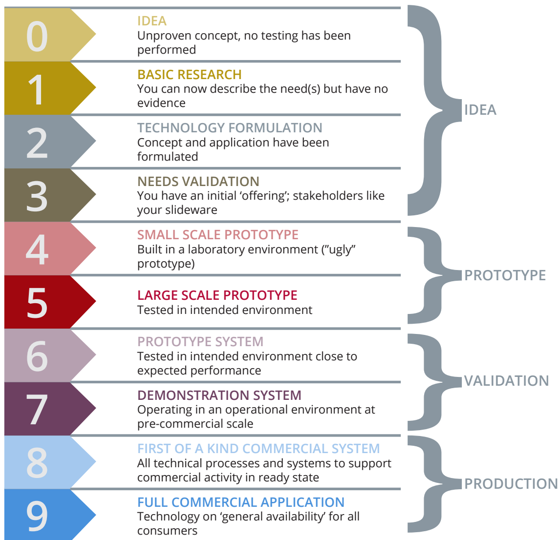
Figure 1: Technology Readiness Levels Source: Technology Readiness Levels, as adapted by the CloudWATCH2
